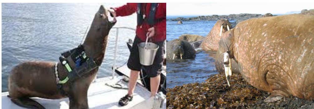
Figure 6. Left panel: Various instruments carried by a Steller sea lion ( Eumetopias jubatus ) using a harness. Right panel: Satellite tag attached with hose clamps to the tusk of a walrus. Photo Left panel: http://www.marinemammal.org ; right panel: Kit Kovacs/Christian Lydersen.
