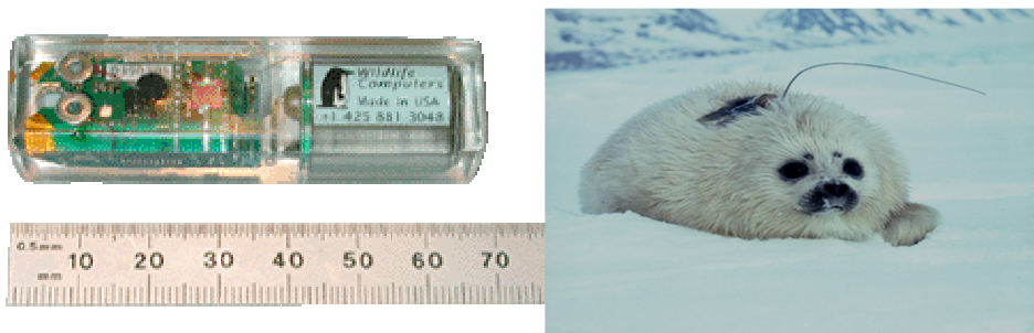
Figure 7. Left panel: A MK-9 Time-Depth Recorder (TDR) from Wildlife Computers. Right panel: A ringed seal pup with a TDR and a VHF transmitter to facilitate recapture. Photo left panel: http://www.wildlifecomputers.com . Right panel: Kit Kovacs/Christian Lydersen.
