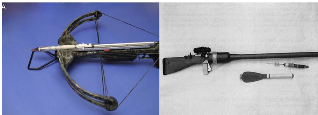
Figure 11. Left panel: a crossbow loaded with an implantable tag and applicator, right panel: Air Rocket Transmitter System (ARTS) consisting of a pneumatic gun, transmitter with steel cutting barbs, and a hollow rocket with tail feathers. Pressure of the compressed air chamber (shown at the base of the barrel of the gun) can be adjusted between 0-50 bar to compensate for distance to target and weight of projectile. Photo: left panel: from Mate et al. 2007, right panel: from Heide-Jørgensen et al. 2001.
