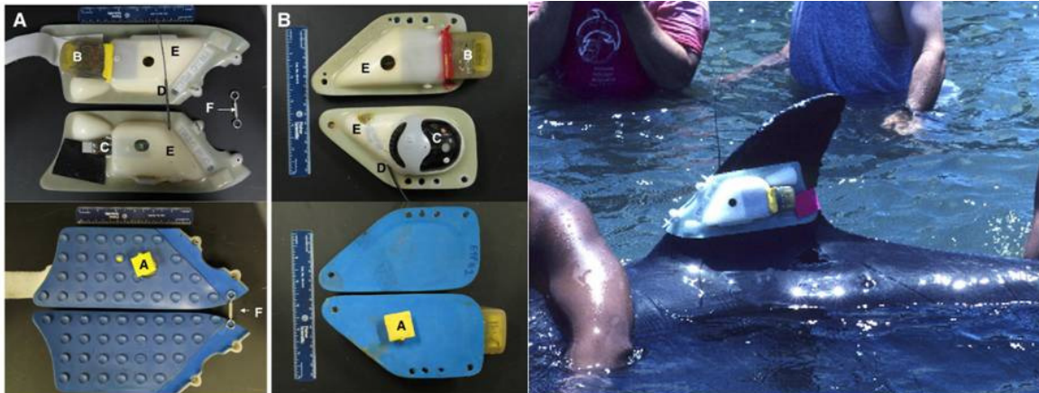
Figure 10. Left panel: (a) a heat flux and skin temperature data logger with suction cup attachment (B) and bolt attachment. Right panel: logger with suction cup attachment on the dorsal fin of an adult bottlenose dolphin. Photo: From Westgate et al. 2007
