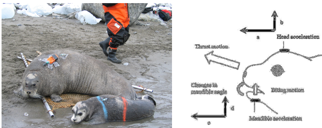
Figure 8. Left panel: An adult bearded seal female with a TDR with incorporated 2-axis accelerometer and camera. This instrument package has a remote release system and will be on the animal for a short time; typically 24 h. The pup has a VHF transmitter to facilitate recapture. Right panel: Schematic drawing showing
