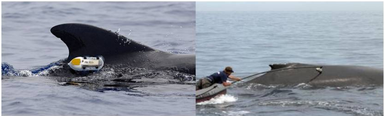
Figure 8. A digital acoustic recording tag (DTAG) attached to a pilot whale (left panel) and a humpback whale ( Megaptera novaeangliae ) (right panel). Photo: left panel: http://www.acousticecology.org/sractiveosonars.html , right panel: http://www.sciencedaily.com/releases/2007/09/070901084549.htm .
