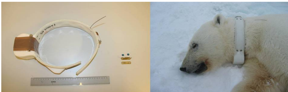
Figure 3. Example of a collar used for satellite tracking of polar bears. Photo: Magnus Andersen.
