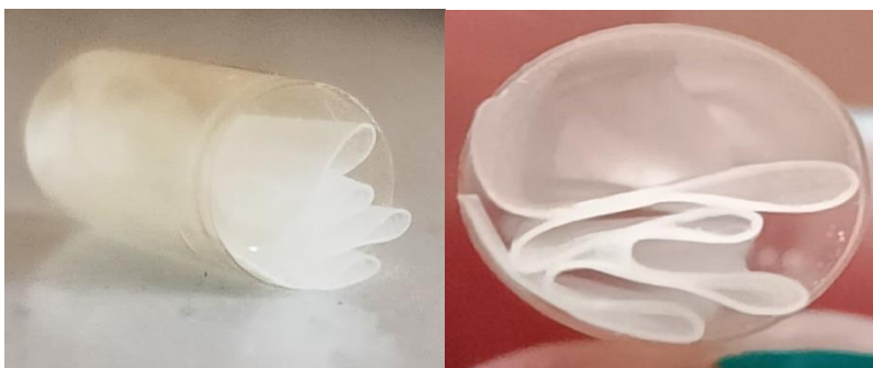
Fig 1 - Film folded in zig-zag pattern and inserted into a capsule shell
