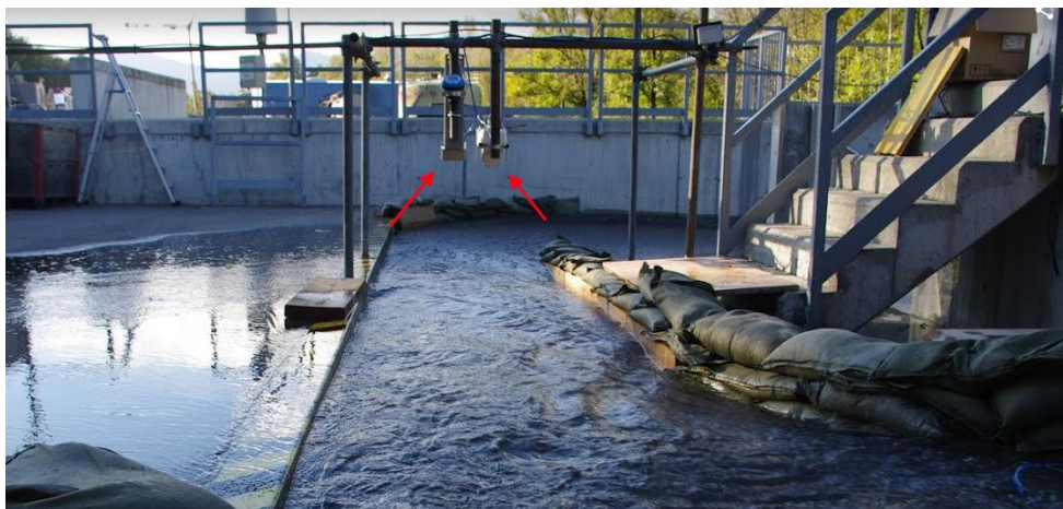
Figure 23: Two radar systems mounted above channel c3: Nivus (left) and Hach (right)
