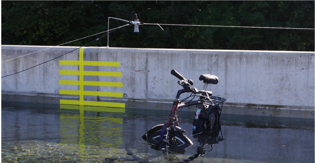
Figure 25: Photo of sensor s3_h_us_maxbotix above storage area s3.
