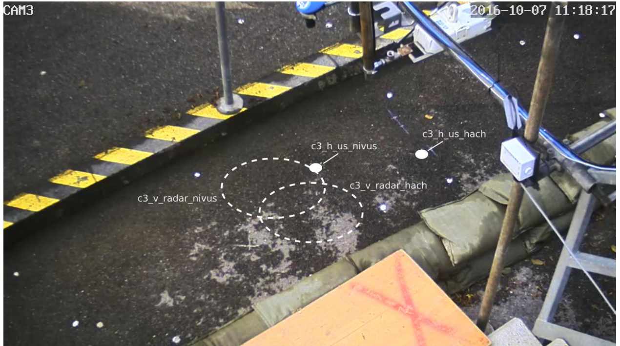
Figure 12: Approximate locations of radar and ultrasonic measurements in image of camera CAM3.
