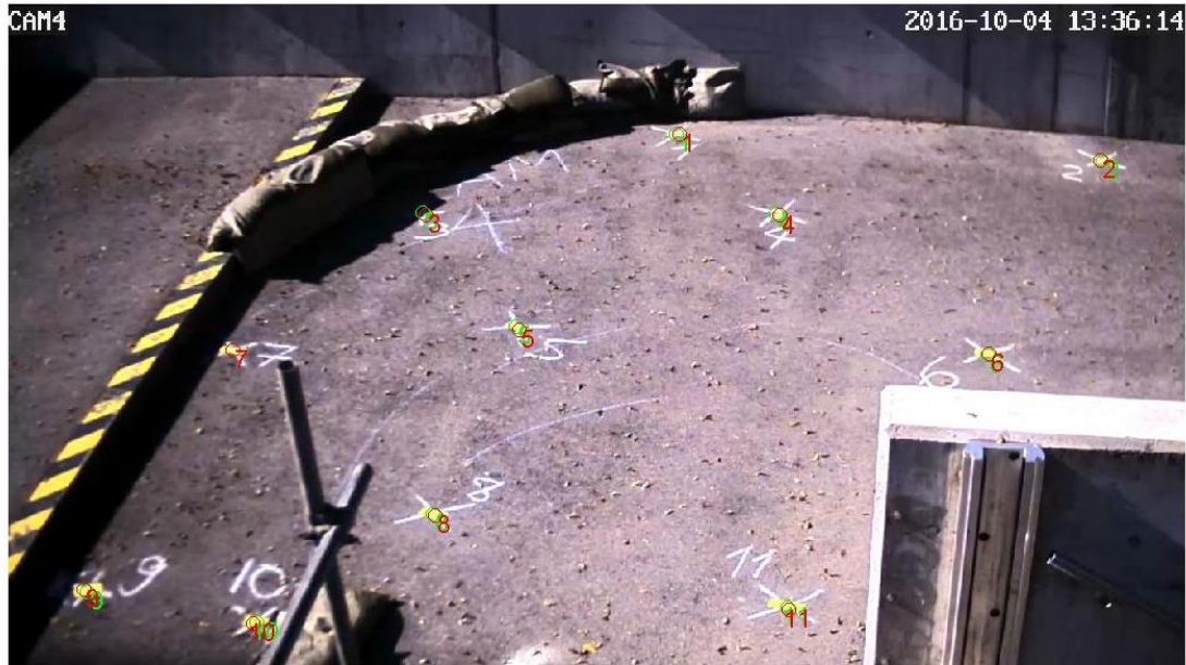
Figure 13: Calibration points and camera parameters of CAM4.
