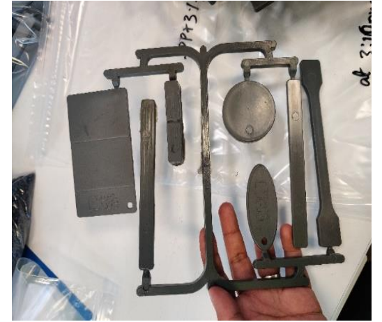
Picture 11 Injection moulded test pieces
