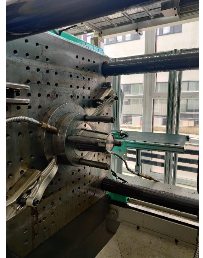
Picture 3. Cup mould on injection moulding machine
