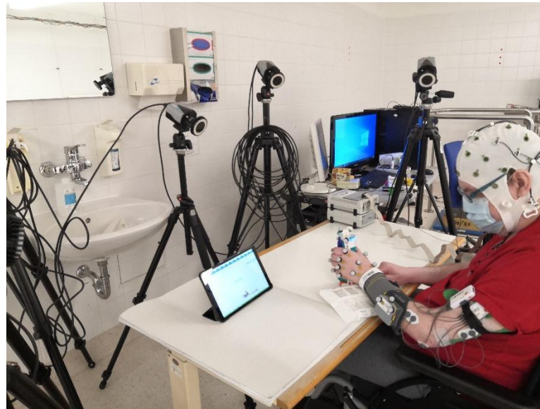
Figure 12. Grasping a sensorized object with support from FES while EEG, EMG and motion capture data is recorded.
