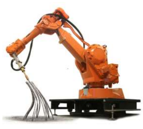
Fig. 3: Shows the Robotic 3D Printer for Bridge Construction. [17]
