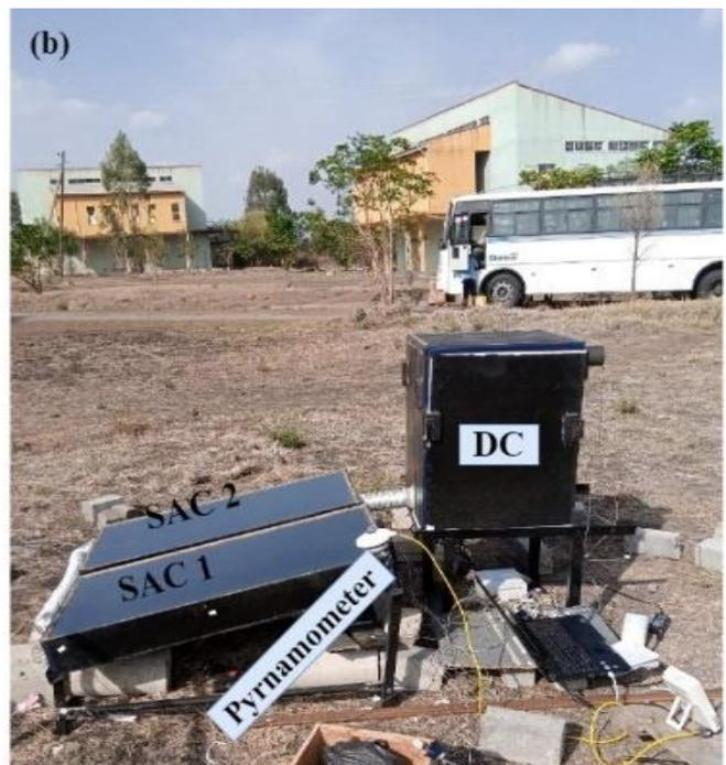
**Figure 4: Schematic (a) and experimental (b) picture of the designed solar dryer.**
