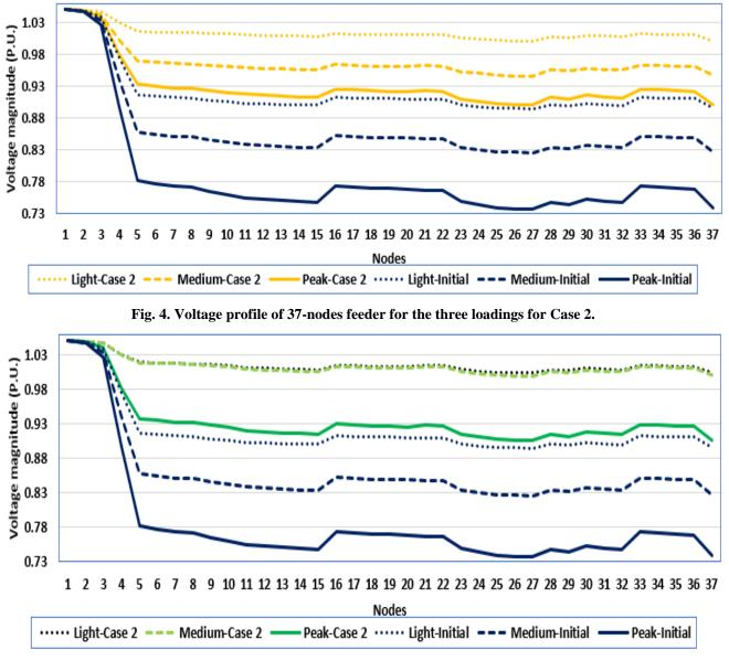
Fig. 5. Voltage profile of 37-nodes feeder for the three loadings for Case 3.
