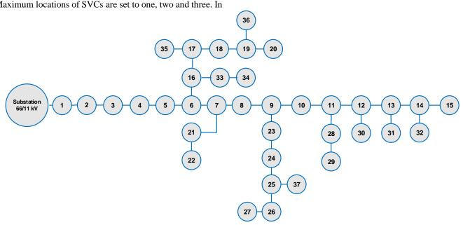
Fig. 1. Single line diagram of 37-node feeder
