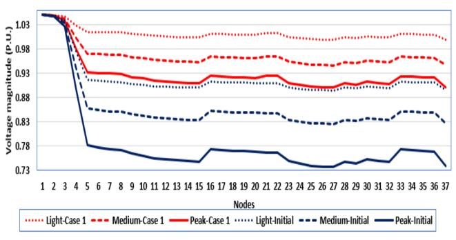
Fig. 3. Voltage profile of 37-nodes feeder for the three loadings for Case 1.
