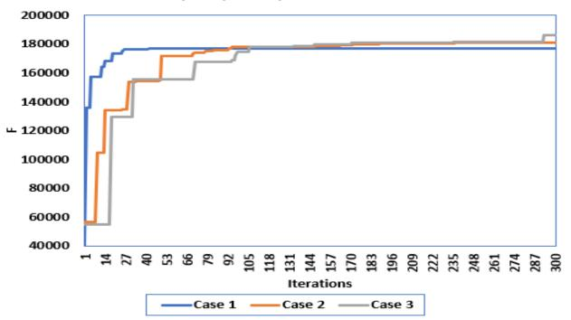
Fig. 2. Convergence characteristics of the differential evolution for the three cases studied.
