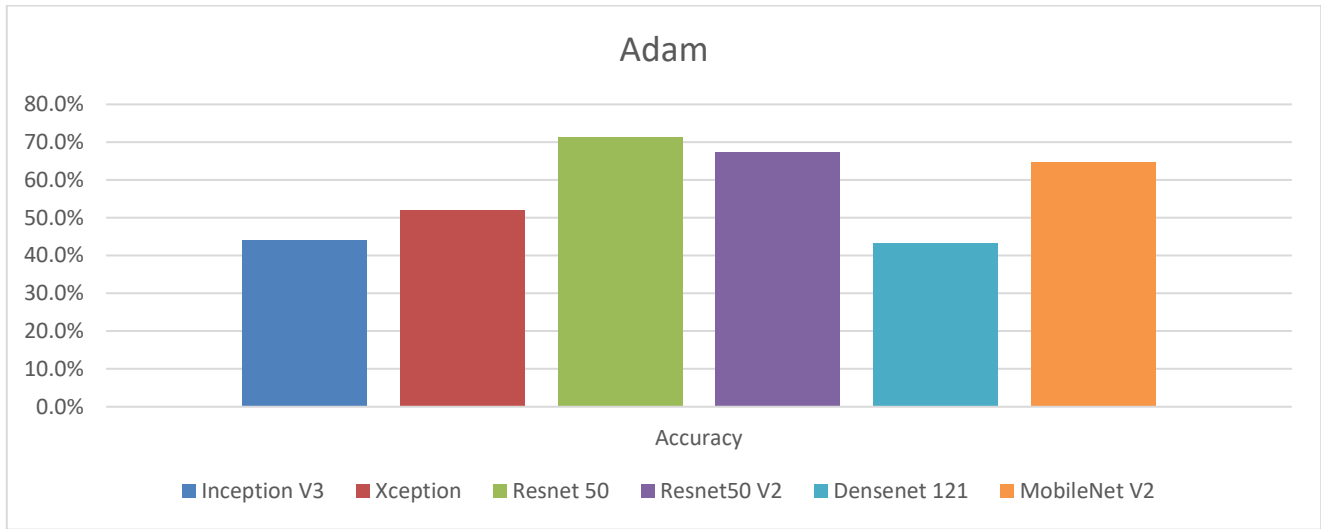
Figure 25. Comparison of accuracy for Adam optimizer for various model with Sigmoid activation function.
