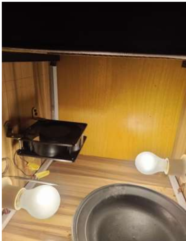
Fig. 7. The bulbs are used to provide heat to the system, while the fan is used to spray the heat across and also help in regulating the temperature of the whole system.
