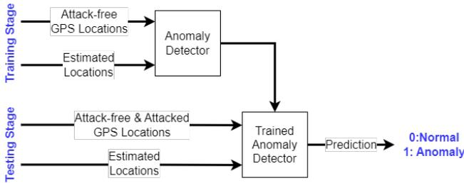
Fig. 2: Machine learning-based anomaly detection pipeline.
