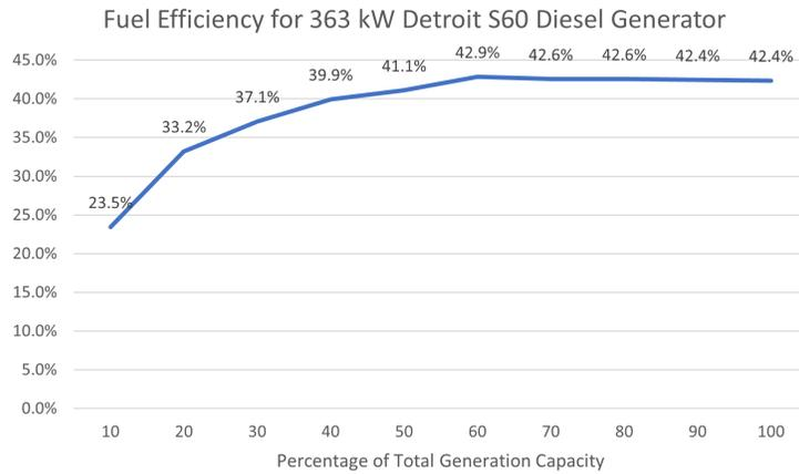
**Figure A.2. Fuel efficiency for 363 kW Diesel Generator model.**
