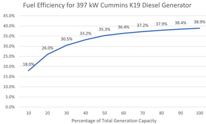
**Figure A.1. Fuel efficiency for 397 kW Diesel Generator model.**
