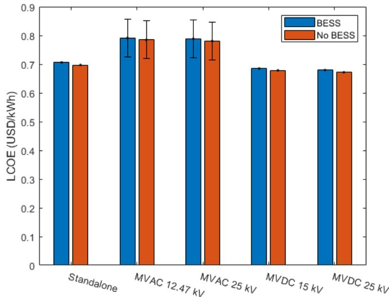
**Figure 1. Modeled Levelized Cost of Electricity of the communities Ambler and Shungnak for the standalone (base case) scenario and the intertie scenarios (MVAC and MVDC) with different line voltages. The MVAC range results from uncertainty of installation costs.**
