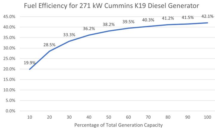
**Figure A.3. Fuel efficiency for 271 kW Diesel Generator model.**
