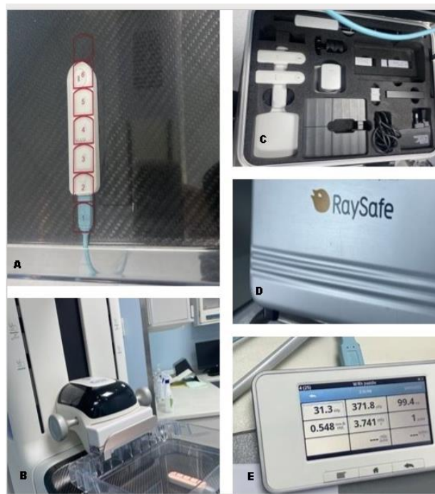
Figure 1: (A) shows the mammography detector, (B) shows detector with compression paddle, (C) shows RaySafe equipment, (D) shows suitcase of RaySafe and (E) shows Unit Base.
