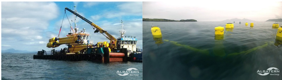
Figure 3 - Deployment of the Albatern Squid devices
