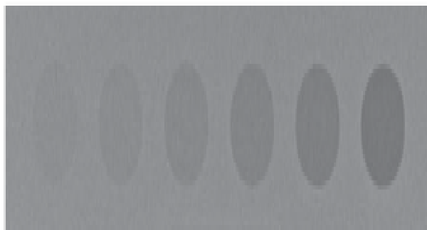
Figure 12: The contrast resolution test. The high contrast resolution should not change over time and should be within the values used in the resolution lead bar. All six low contrast objects should be visible and should not change over time.
