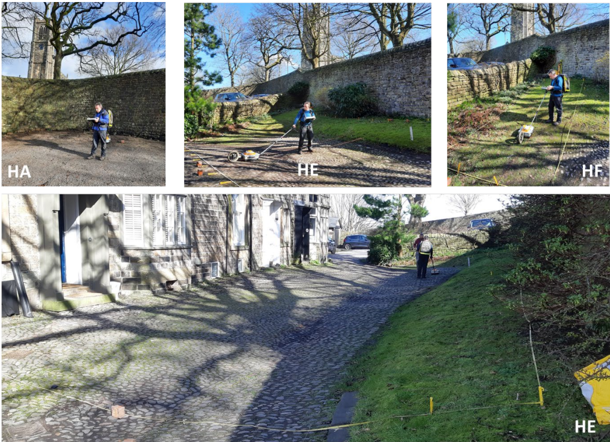
Figure 8: Site photographs taken during 500MHz GPR surveys.
