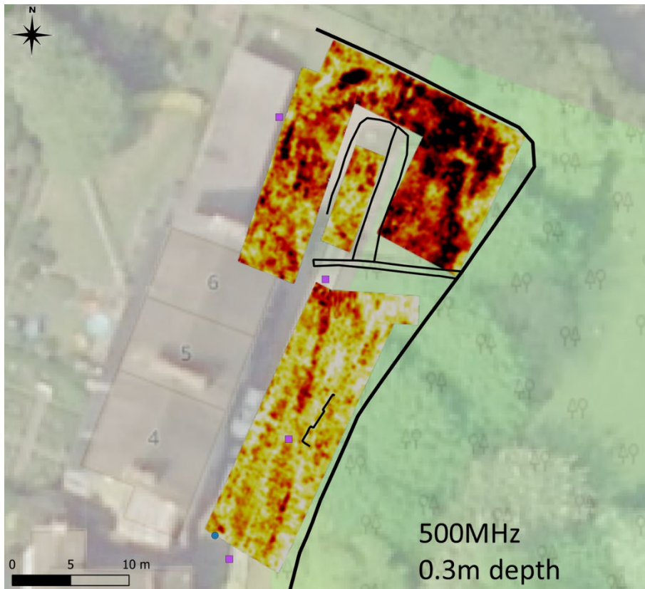
Figure 9: Horizontal slice of 500MHz GPR model at 0.3m below ground level. Darker colours indicate stronger reflected signals.
