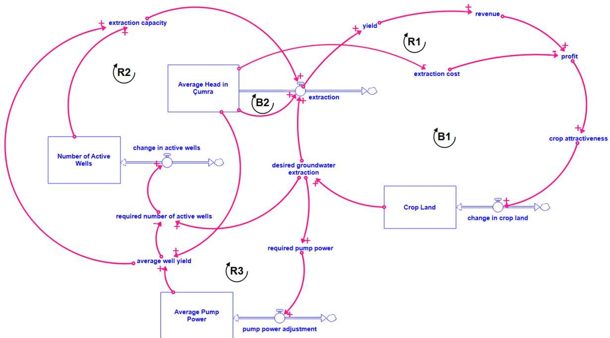
Figure 1. The main feedback overview of the model
