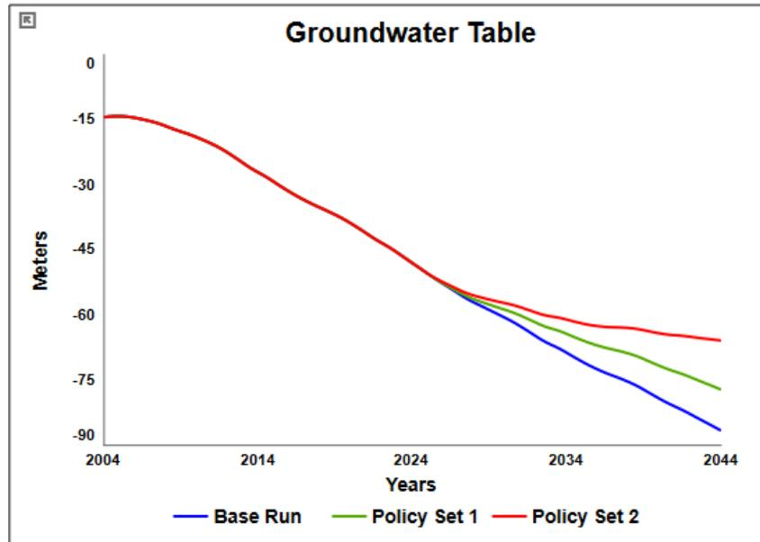
Figure 28. Integrated policy analysis 1: Groundwater level
