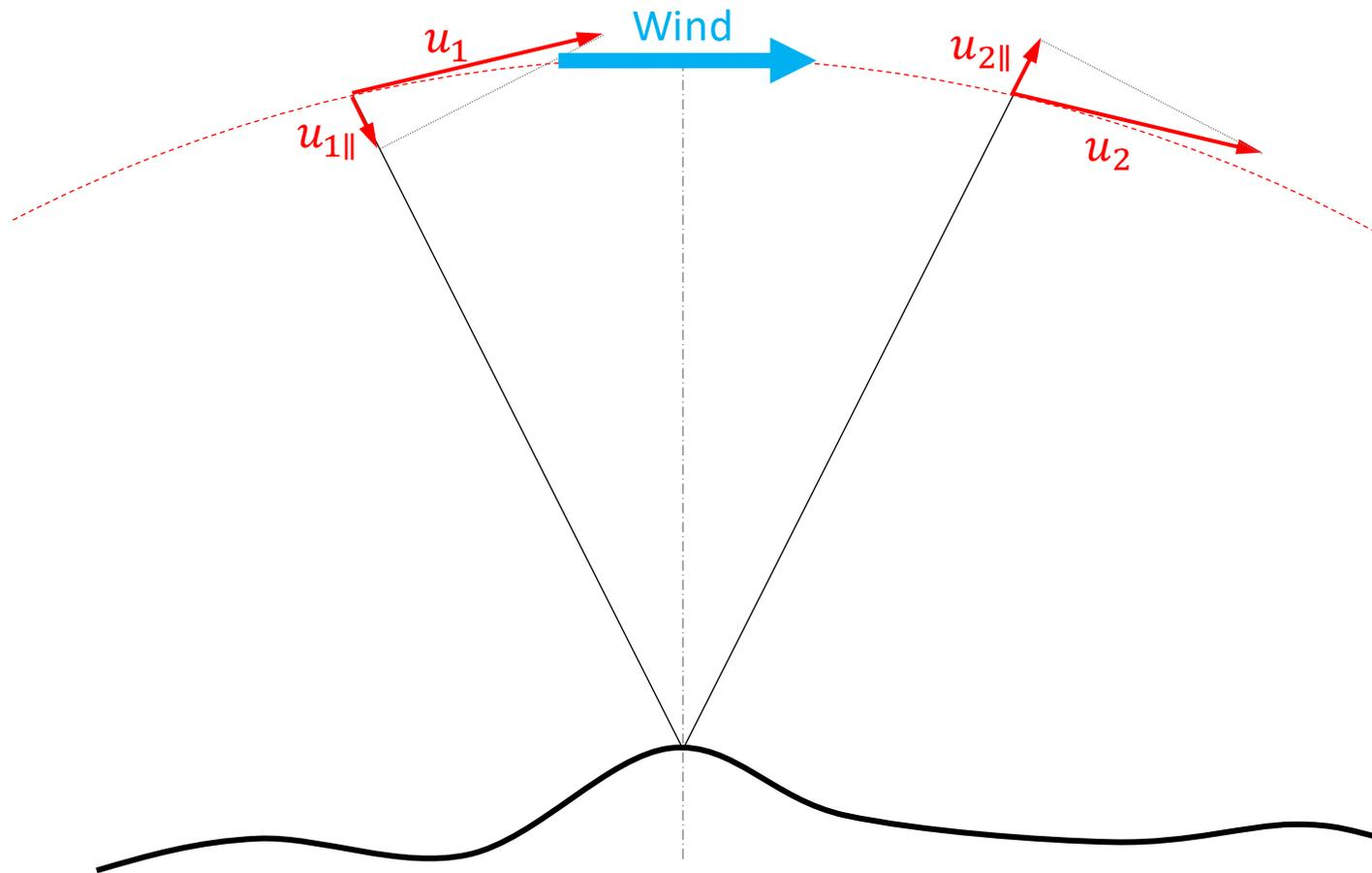
Different wind speeds with different flow geometries give same measurement result.
