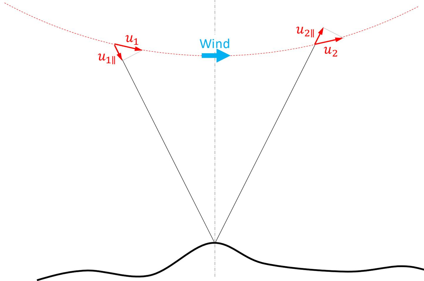
Different wind speeds with different flow geometries give same measurement result.
