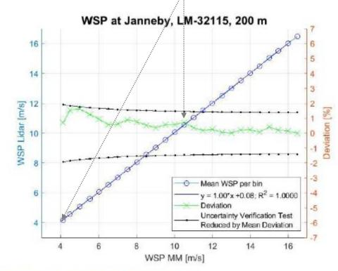
Figure 14: Scatterplot bin-wise wind speed and deviation at 200 m
