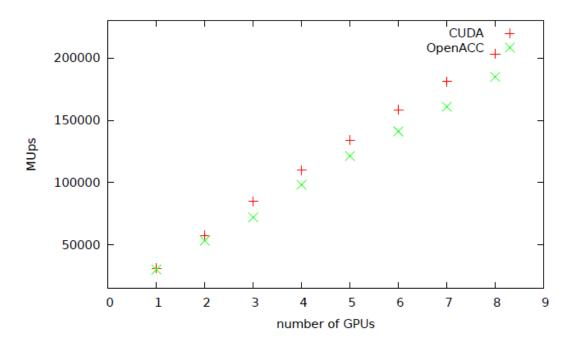
Figure 7 The weak scaling on a node with 8 NVIDIA M2090 cards.
