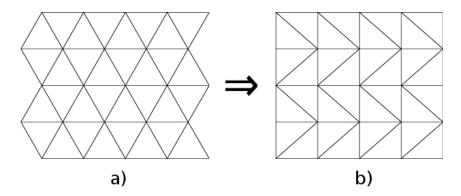
Figure 3 A triangular lattice (a) can be mapped onto a rectangular lattice by shifting every second row by half the lattice constant (b).
