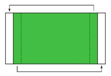
Figure 4 A schematic of periodic boundary conditions. Each edge column is mirrored in an extra column added on the other side of the grid.
