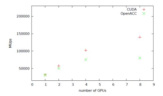
Figure 6 The strong scaling on a node with 8 NVIDIA M2090 cards.
