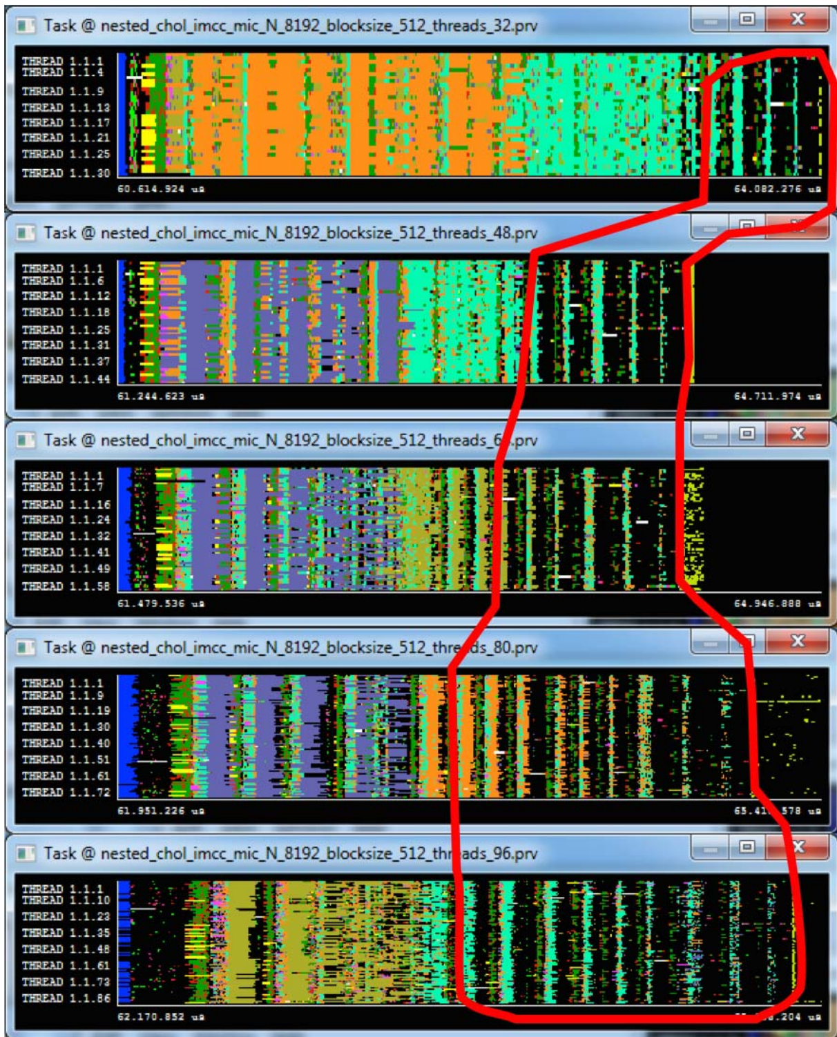
Figure 12. Trace file of Cholesky (OmpSs with nesting) with 32, 48, 64, 80 and 96 hardware threads
