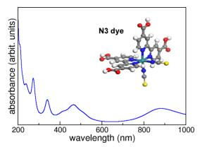
Numerical details: Number of atoms = 59, number of electrons= 218, cell=(19.0x19.0x19.0)Å<sup>3</sup>, Ecut=25Ry, FFT=(192x192x192), XC=PBE, USPP..
