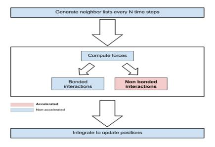
Figure 1: GROMACS compute-flow diagram. Adopted from [11].
