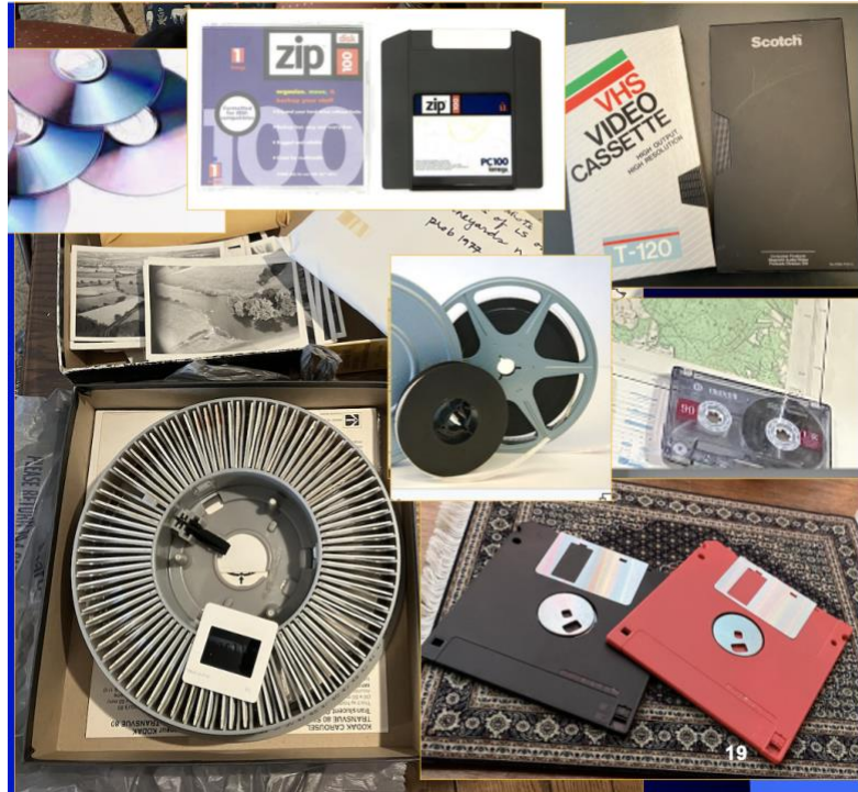
Figure 3 - Data from our project in its many, outdated formats such as 35 mm slides, floppy drives, audio cassettes, Super 8 mm movie film, VHS videos, CD-ROMs, and Zip disks, none of which are supported today.
