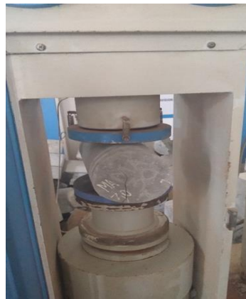
Fig.2:-Split Tensile Strength Test
