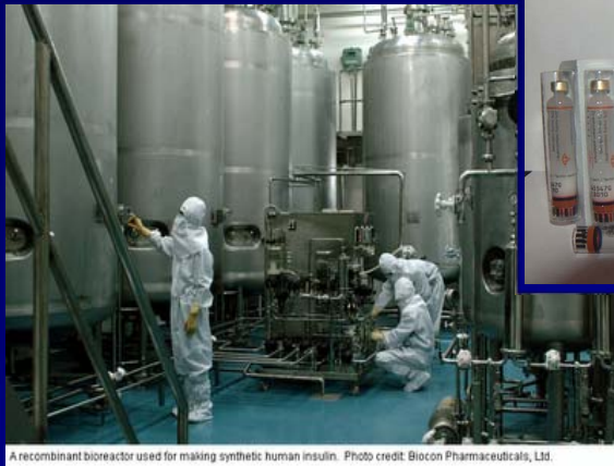
A recombinant bioreactor used for making synthetic human insulin. Photo credit: Biocon Pharmaceuticals, Ltd.
