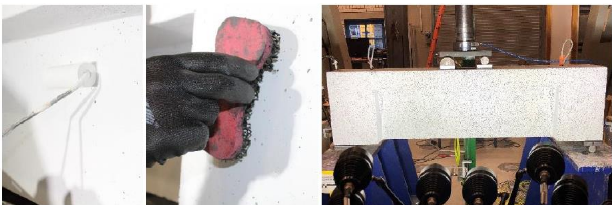
Figure 3: Priming (left), applying the pattern (middle) and prepared beam with stochastic pattern
