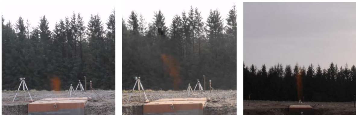
Figure 3-6 Visibility of hydrogen fires in 8-inch steel pipes under pressures of (from left to right) 350 mbar, 2 bar and 7 bar and without ground cover [26] [27]
