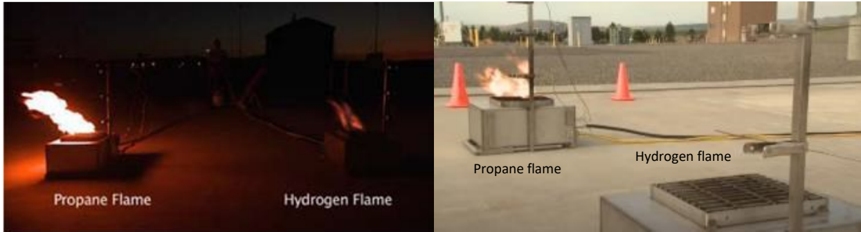
Figure 3-4 A propane flame and hydrogen flame at night (left) and during the day (right) [22]
