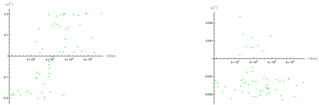
Figure 38: The Error Distribution of \delta of Asteroids with Respect to Their Distance From the Spacecraft, Error of the RF is not included on the left - included on the right.
