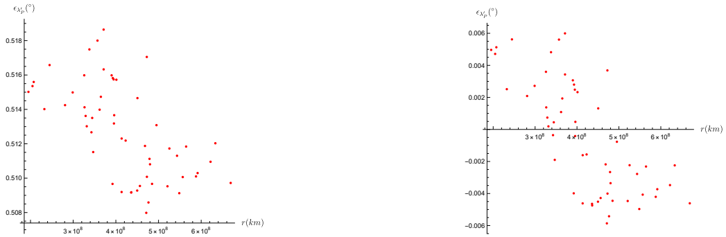
Figure 155: The Error Distribution of \lambda'_p of Asteroids with Respect to Their Distance From the Spacecraft, Error of the RF is not included on the left - included on the right.
