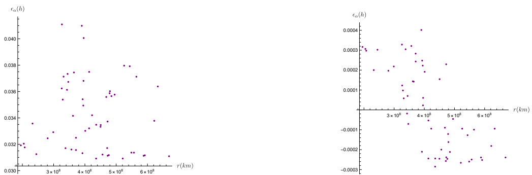
Figure 97: The Error Distribution of \alpha of Asteroids with Respect to Their Distance From the Spacecraft, Error of the RF is not included on the left - included on the right.
