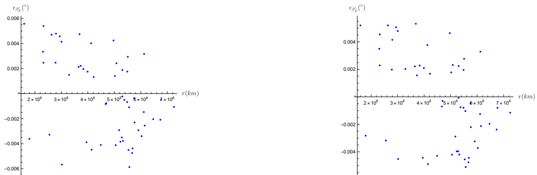
Figure 60: The Distribution of Error in \beta'_p of Asteroids with Respect to Their Distance From the Spacecraft, Error of the RF is not included on the left - included on the right.
