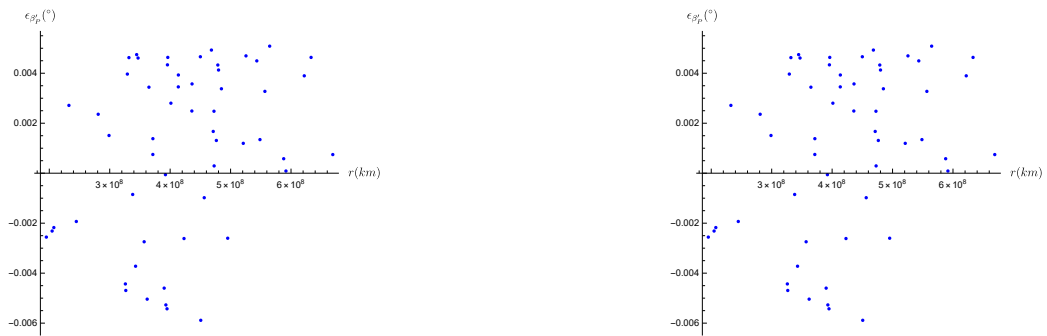
Figure 216: The Error Distribution of \beta'_p of Asteroids with Respect to Their Distance From the Spacecraft, Error of the RF is not included on the left - included on the right.
