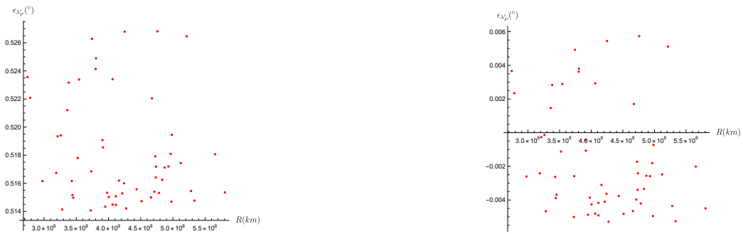
Figure 114: The Distribution of \lambda'_p Error of Asteroids with Respect to Their Distance From the Sun, Error of the RF is not included on the left - included on the right.
