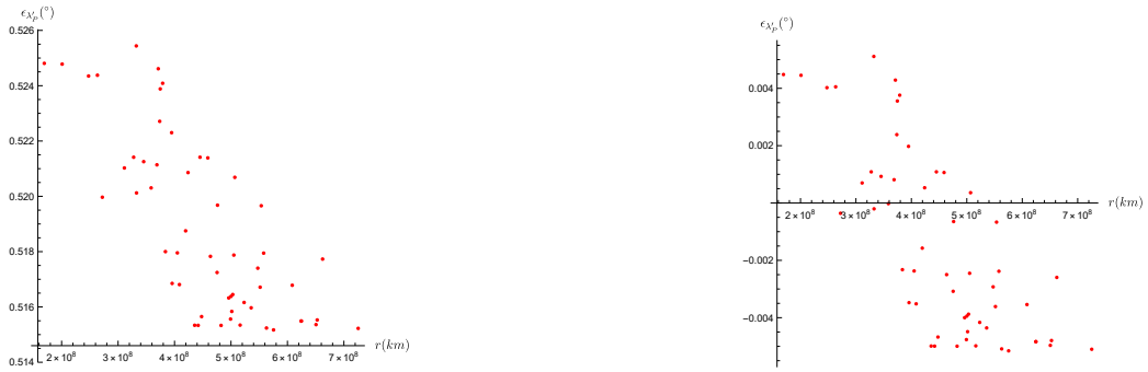
Figure 47: The Error Distribution of \lambda'_p of Asteroids with Respect to Their Distance From the Spacecraft, Error of the RF is not included on the left - included on the right.
