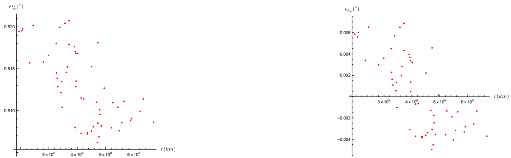
Figure 95: The Error Distribution of \lambda'_p of Asteroids with Respect to Their Distance From the Spacecraft, Error of the RF is not included on the left - included on the right.
