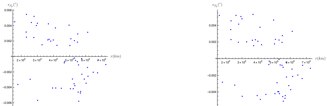
Figure 180: The Distribution of Error in \beta'_p of Asteroids with Respect to Their Distance From the Spacecraft, Error of the RF is not included on the left - included on the right.
