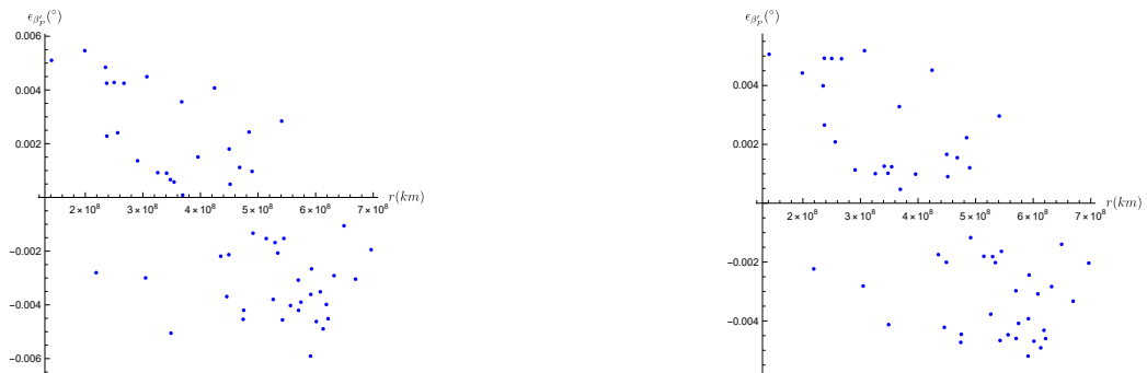
Figure 132: The Distribution of Error in \beta'_p of Asteroids with Respect to Their Distance From the Spacecraft, Error of the RF is not included on the left - included on the right.
