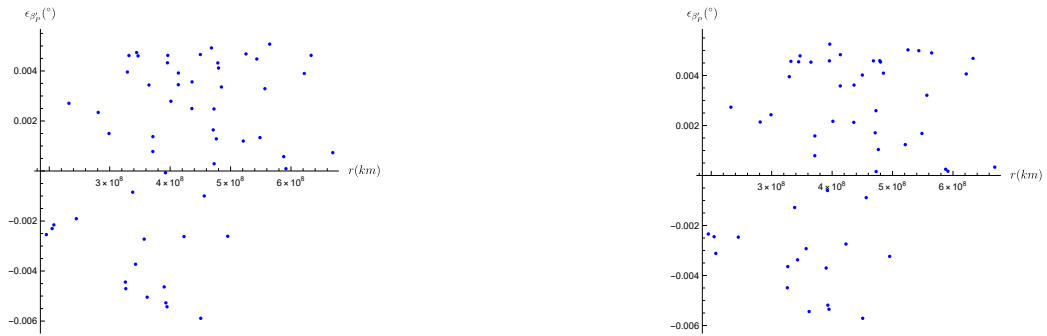
Figure 156: The Error Distribution of \beta'_p of Asteroids with Respect to Their Distance From the Spacecraft, Error of the RF is not included on the left - included on the right.
