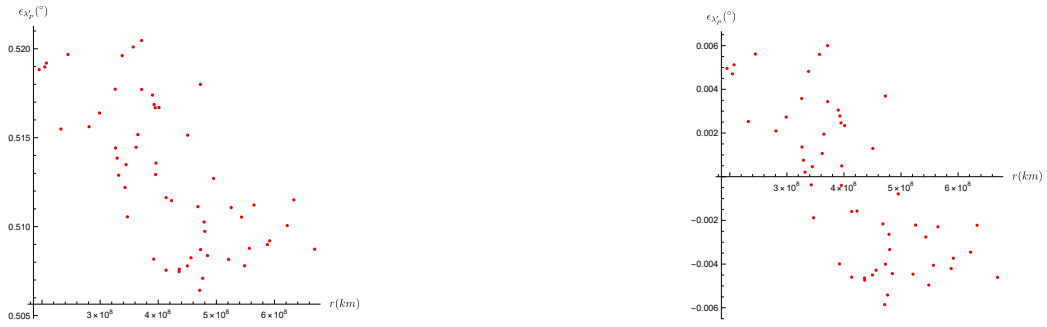
Figure 35: The Error Distribution of \lambda'_p of Asteroids with Respect to Their Distance From the Spacecraft, Error of the RF is not included on the left - included on the right.
