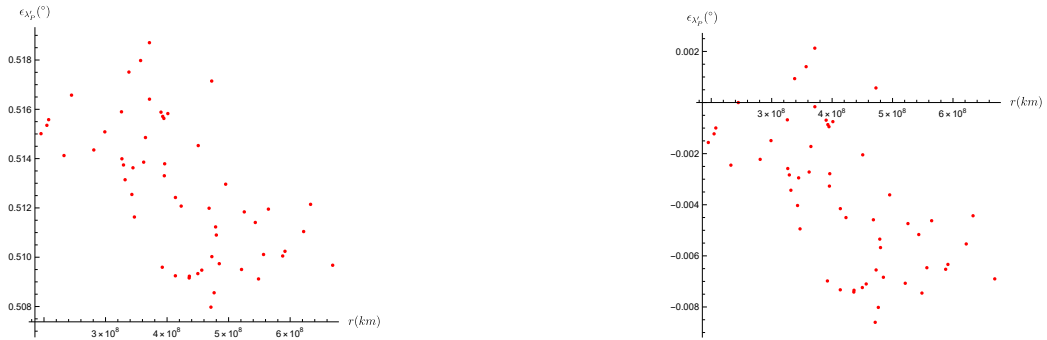
Figure 215: The Error Distribution of \lambda'_p of Asteroids with Respect to Their Distance From the Spacecraft, Error of the RF is not included on the left - included on the right.
