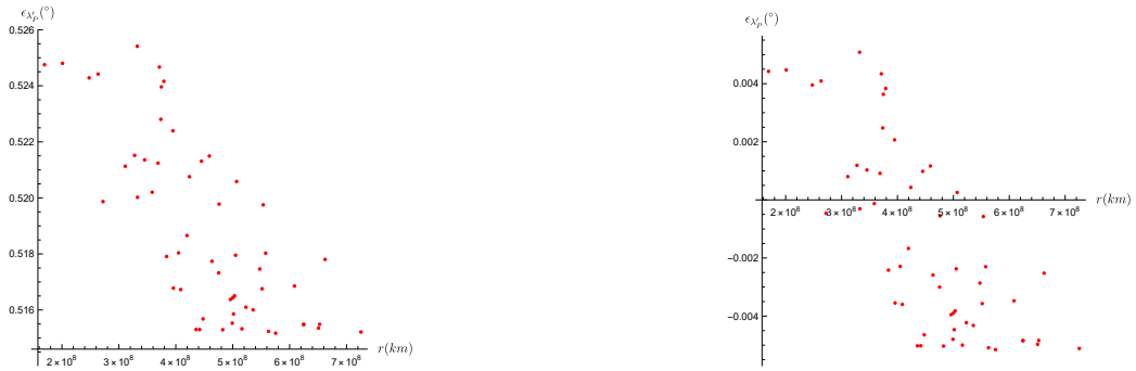
Figure 227: The Error Distribution of \lambda'_p of Asteroids with Respect to Their Distance From the Spacecraft, Error of the RF is not included on the left - included on the right.
