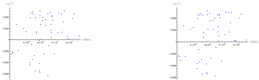
Figure 96: The Error Distribution of \beta'_p of Asteroids with Respect to Their Distance From the Spacecraft, Error of the RF is not included on the left - included on the right.
