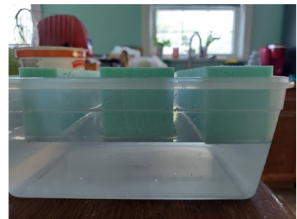
(b) Foam block floating in a water with density ratio of around 0.05.
