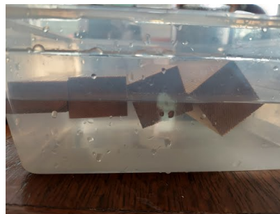
(a) Wooden block floating in a water with density ratio of around 0.6.
