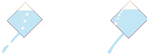
Fig. 16.12 – Counter-current flow in a can (the left figure) has only one hole thus pulse flow and a flow with two holes (right picture).
