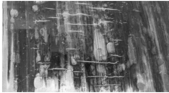
Figure 4. Brake pulley friction surface with microcracks and partial thermal spots.
