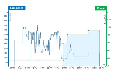
Figure 1 (Indoor Luminance Levels (volatile line) vs Manual Control Actions (step-wise line).
