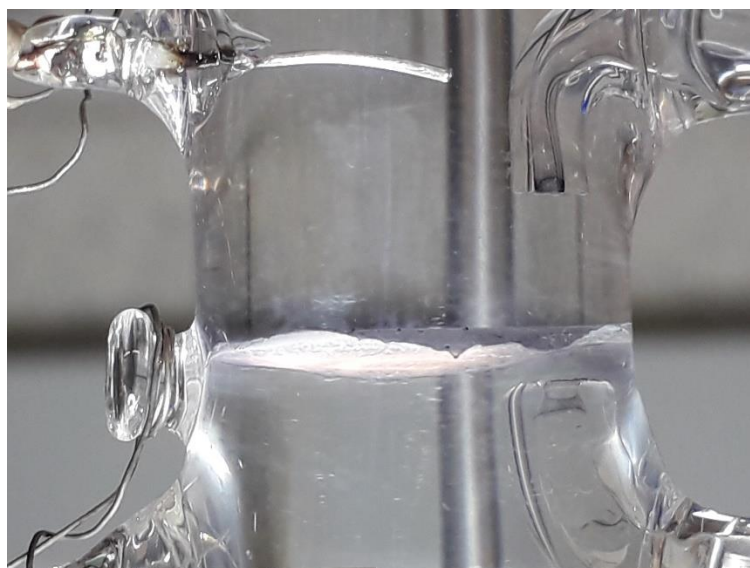
Figure S7. Optical image of the white underside (or organic-facing side) of a free-floating AuNP/poly(DMcT) interfacial film after all remaining colloidal AuNPs in the bulk aqueous phase were extracted by thoroughly rinsing with a colloidal AuNP-free aqueous electrolyte solution ( e.g. , 10 mM LiCl).
