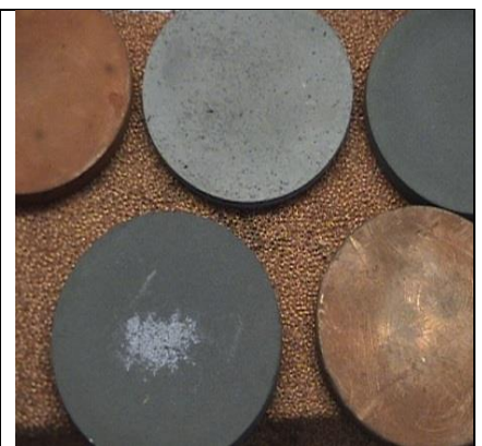
Figur 3. Metal-ceramic filter elements obtained by the method of CVD impregnation of porous structures.
