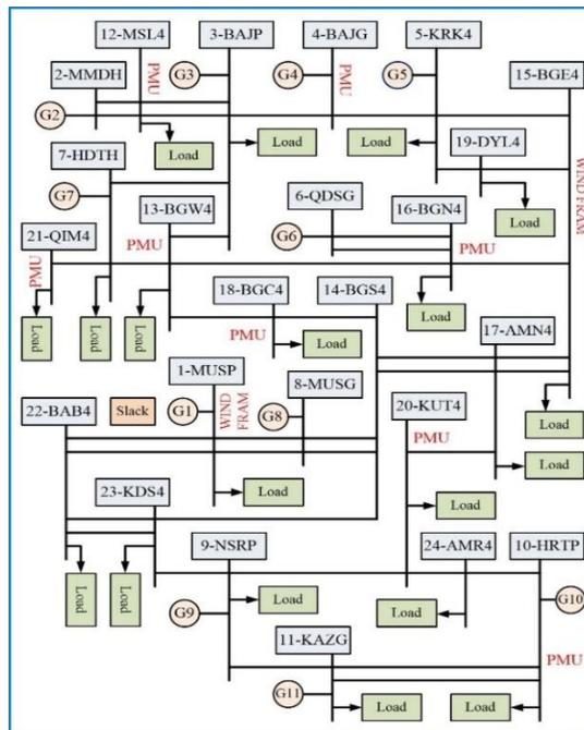
Figure 2. Iraqi power system single line diagram with PMU installation and wind farms [23]
