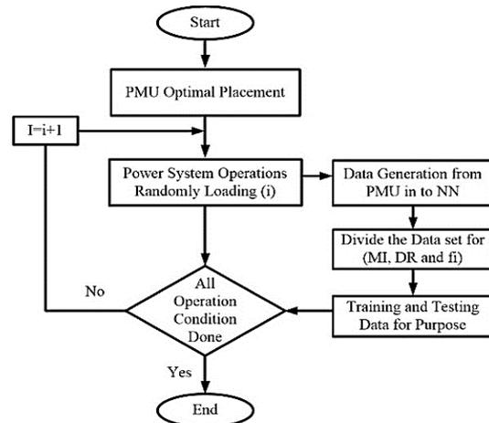
Figure 5. Flow chart of PMU-NN algorithm-based monitoring system
