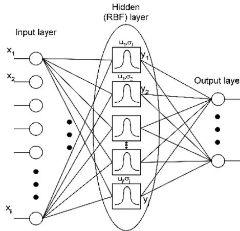
Figure 3. Radial basis function neural network (RBFNN) [4]
