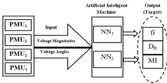
Figure 4. Block diagram for PMU-NN monitoring system
