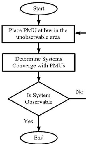
Figure 1. Flowchart of the GTPA PMU placement [21]–[23]
