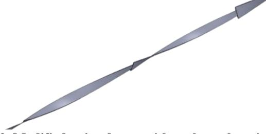
Fig 2. Modified twisted tape without lateral projection
