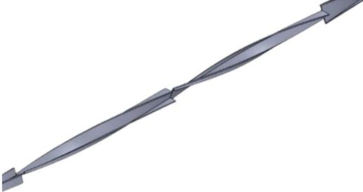
Fig 3. Modified twisted tape with lateral projection
