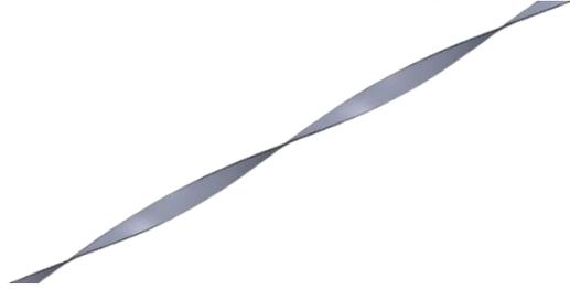
Fig 1. Geometry of conventional twisted tape
