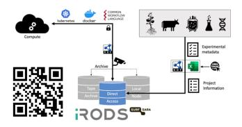
Figure 2. FAIR data platform technical details. Experiment metadata is used to program the iRODS DMS to store data in designated folders along with the metadata. Data transformation and analysis is done using containerized applications. Kubernetes is used manage container deployment. QR-code: https://m-unlock.nl
