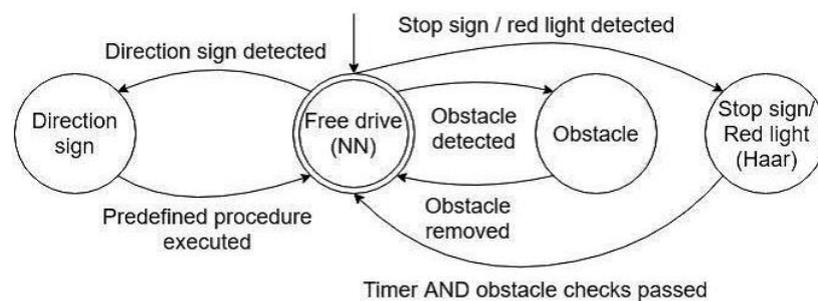
**Figure 4.** Autonomous mode finite state machine
