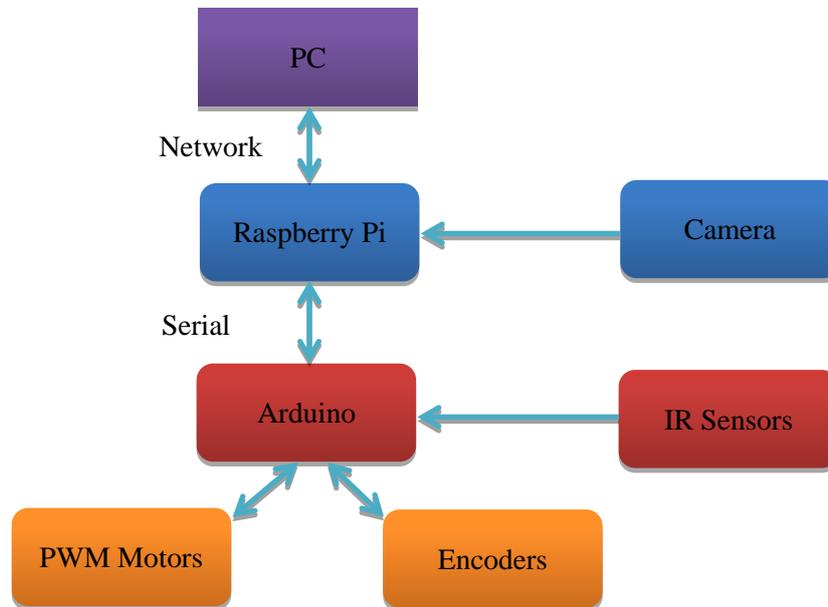
**Figure 2.** Connections of the electrical components of the system
