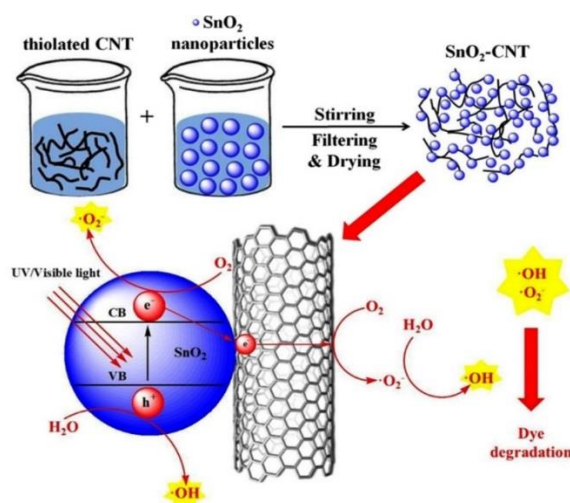
Figure 2. Schematic diagram of the preparation process of SnO 2 /CNT NNs composites [23]
