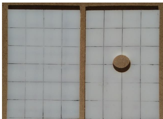
Figure 2: Hammer hit points defined on rectangular plates.
