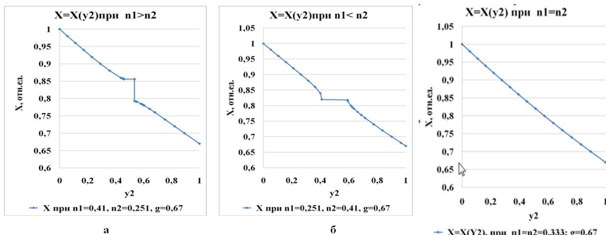
1 rasm. Ikki fazali geterogen muhit nisbiy samaraviy o‘tkazuvchanligi ( $X$ )ning past o‘tkazuvchanlikli fazaning hajmiy ulushi  $y_2$ ga nisbatan bog‘lanishi ( $g=0,67$ ): a -  $\text{Bi}_2\text{Te}_3\text{-Sb}_2\text{Te}_3$  aralashma uchun ( $n_1=0,41$ ;  $n_2=0,251$ ). b -  $\text{Bi}_2\text{Te}_3\text{-Sb}_2\text{Te}_3$  aralashma uchun ( $n_1=0,251$ ;  $n_2=0,41$ ). v -  $\text{Bi}_2\text{Te}_3\text{-Sb}_2\text{Te}_3$  aralashma uchun ( $n_1=0,333$ ;  $n_2=0,333$ ) hisoblangan natijalar.
