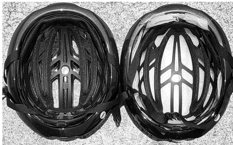
Figure 1: Left: Standardized bicycle helmet (EPS Foam); Right: Modified Bicycle Helmet (Polyolefin Foam).
