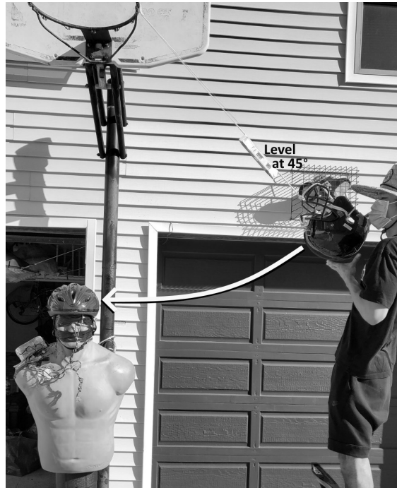
Figure 2: Simulation model setup showing the weighted football helmet and the manikin wearing the bicycle helmet.
