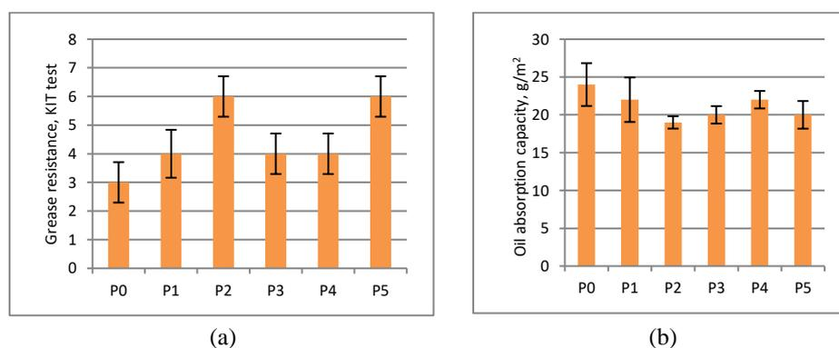
Fig. 5 – The oil and grease barrier properties of xylan coated papers.
