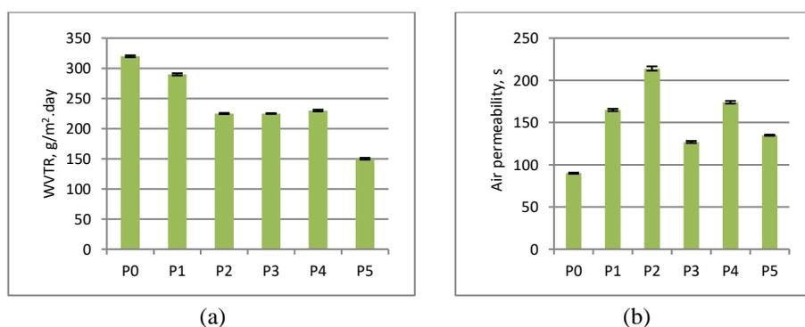
Fig. 4 – The water vapour and air barrier properties of xylan coated papers.
