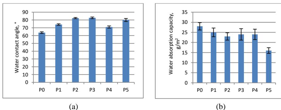
Fig. 3 – The water barrier properties of xylan coated papers.
