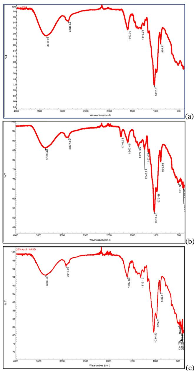
Fig. 1 – FT-IR spectra of (a) hardwood xylan (Xy); (b) acetylated xylan (XyAc); (c) AKD hydrophobized xylan (XyAKD).
