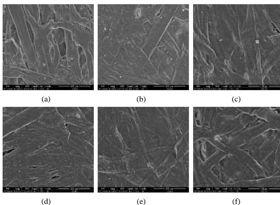
Fig. 2 – SEM images of coated paper samples with xylan and xylan derivatives: (a) P0 -base paper; (b) P1- Xy coated paper in single layer; (c) P2 -XyAKD coated paper in single layer; (d) P3 -XyAc coated paper in single layer; (e) P4 –layered coated paper: 2Xy; (f) P5 -Layered coated paper: base layer of Xy; top layer of XyAKD.
