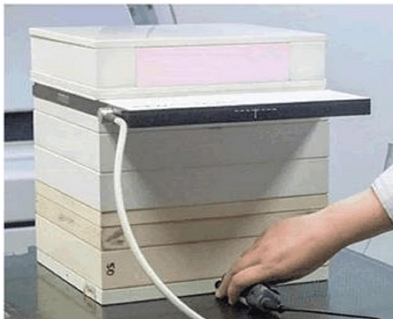
Figure 1: The initial evaluation setup utilizing an ionization chamber.
