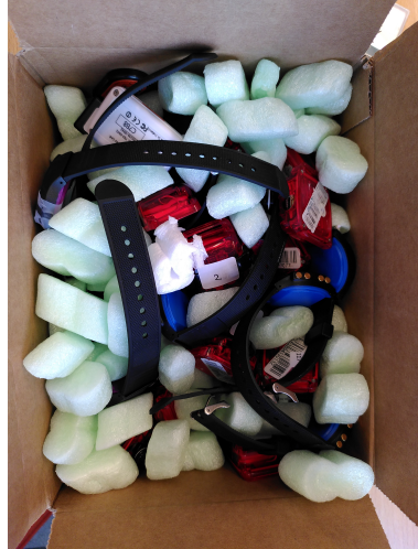
Figure 3: Accelerometers placed in a cardboard box during the box experiment.
