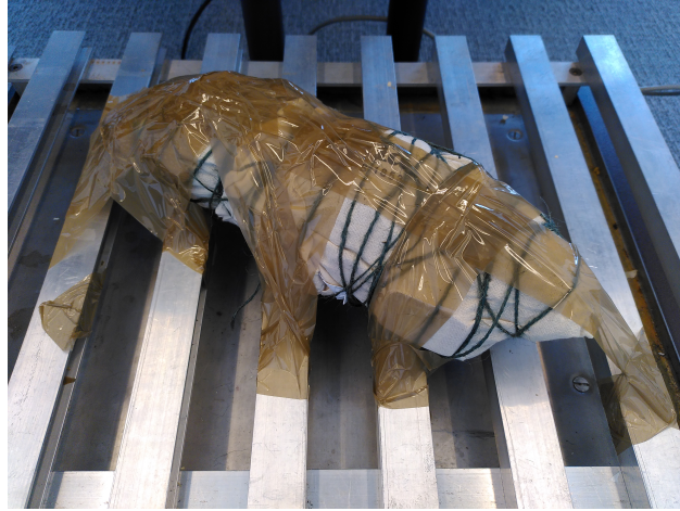
Figure 2: Attachment of the accelerometers in the bag to the mechanical shaker machine during the ms_bag experiment.
