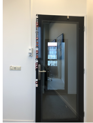
Figure 4: Attachment of a subset the accelerometers during the door experiment.
