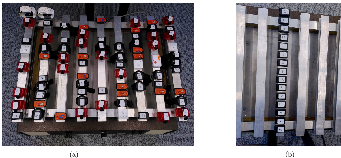
Figure 1: Attachment of the accelerometers to the mechanical shaker machine during the ms_lrcr , ms_hrcr and ms_mrcr (a) and ms_lrmr and ms_hrmr (b) experiments.
