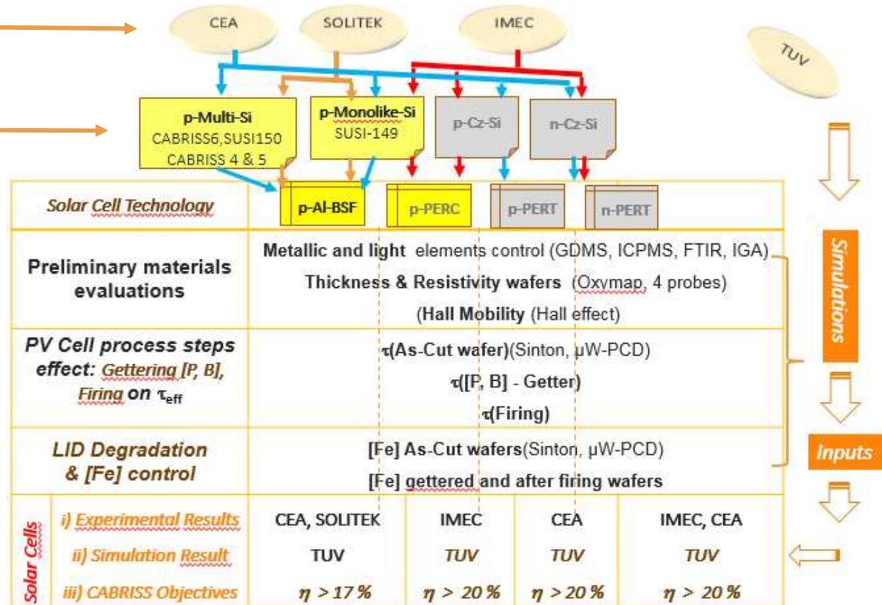
We propose an overall protocol to qualify Re-Si wafers coming from different ingots & different Re-Si feedstock and to evaluate their potential in the different solar cell technologies.
