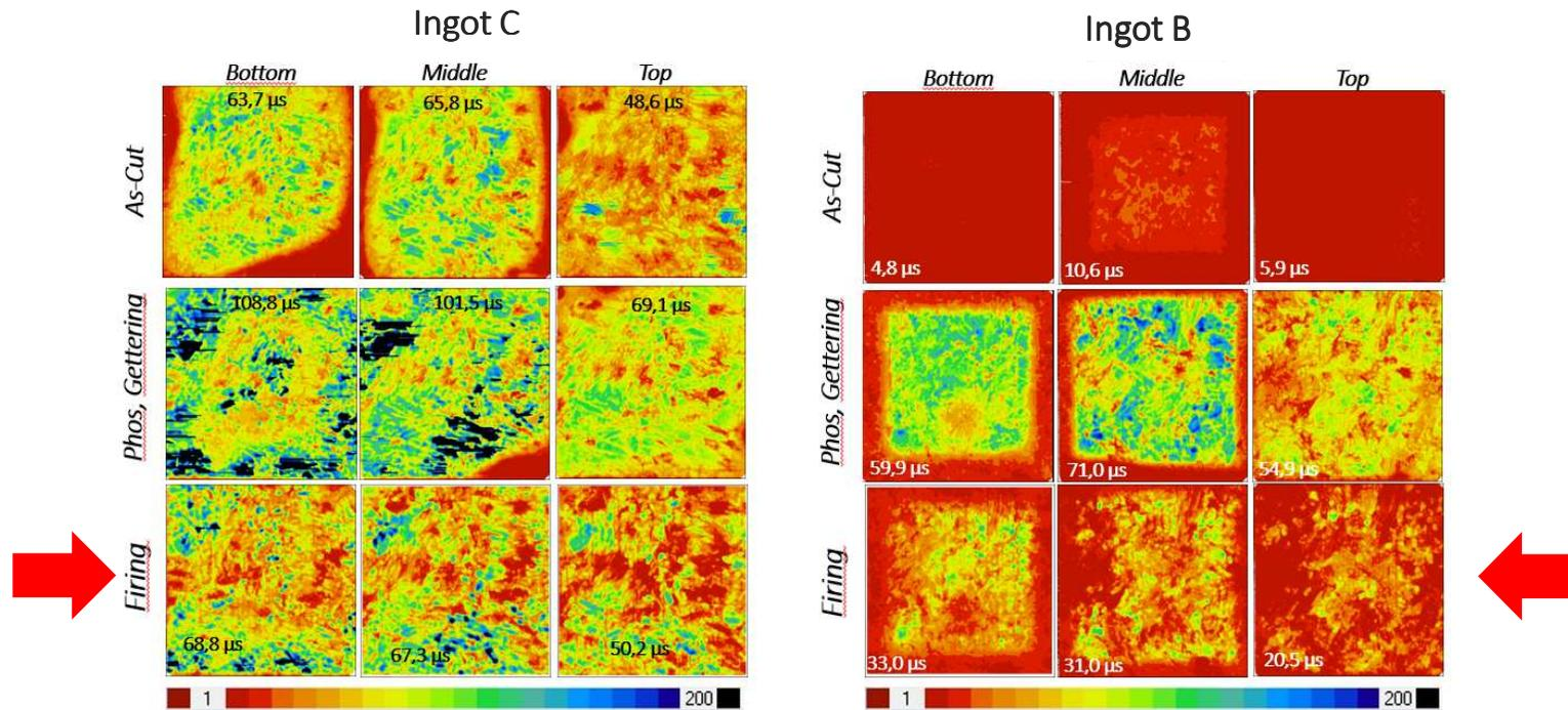
The  $\mu$ WPCD mappings confirm the degradation of the gettered wafers after firing step. We have to notice that this effect will be reduced for solar cell due to the presence of phosphorus emitter[1]
