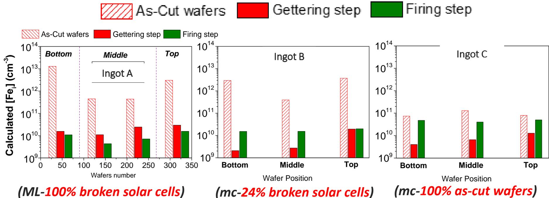
The higher the amount of the Re-Si broken solar cells feedstock, the higher  $[Fe_i]$  content in as-cut wafers.
