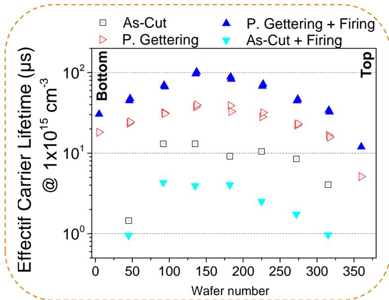
Good agreement between Characterization Protocol and Al-BSF solar cells on ingot A wafers.
