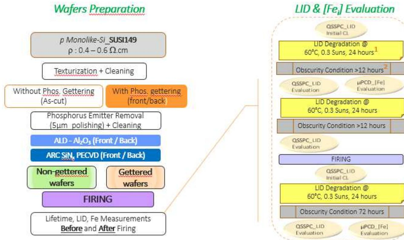
In order to evaluate Re-Si wafers electrical quality,  $\tau_{\text{eff}}$  of (as-cut, P gettered and after firing wafers), were measured with QssPC and  $\mu\text{W-PCD}$  instruments during Al-BSF process.
