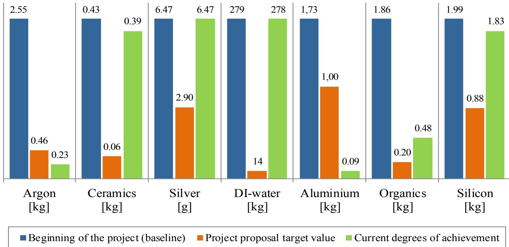
*Reduction of waste and resource consumption per production unit for mono-Si based PV-module (60 6-inch solar cells) envisaged at the beginning of the project and current degrees of achievement*
