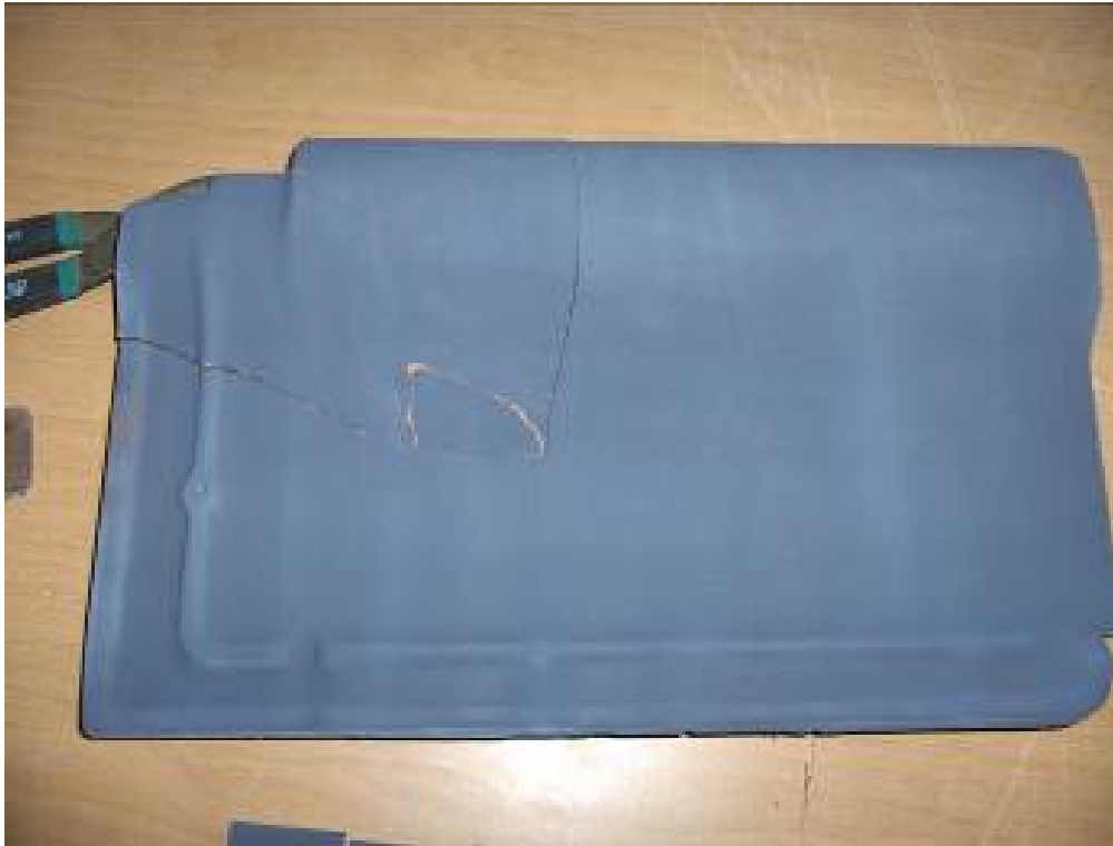
A ceramic roof tile, fully covered with Al/Si coatings
