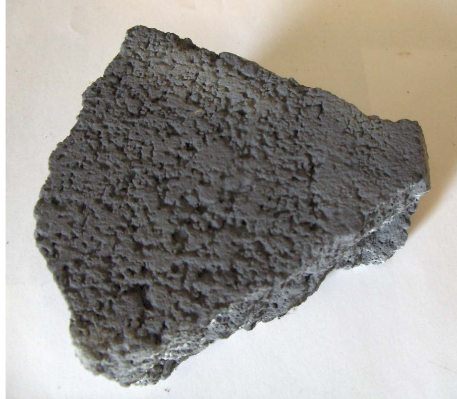
Si coating on concrete
