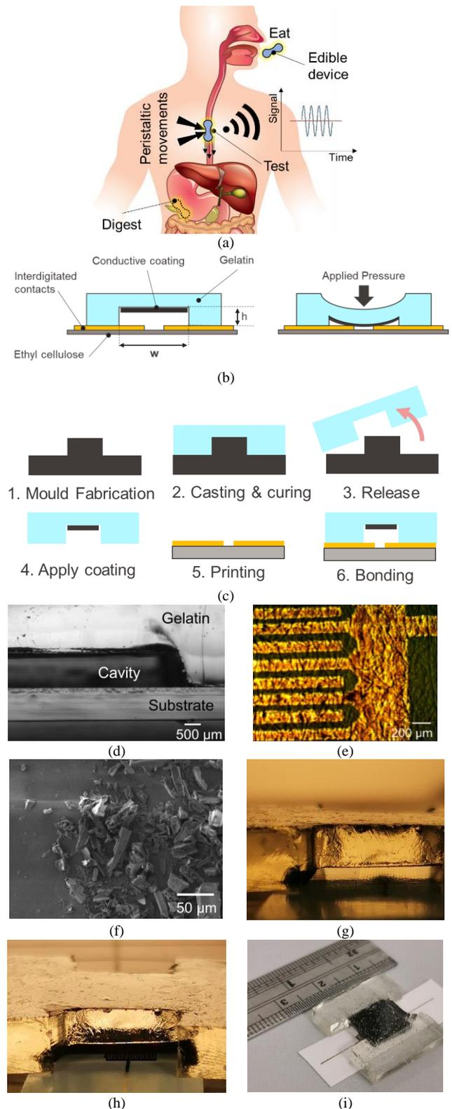
Fig. 1. (a) Application scenario. (b) Working principle of the edible resistive pressure sensor. (c) Fabrication method of the sensor. (d) Section of the gelatin/glycerol microstructure ( $h = 1$  mm). (e) Micrograph of the interdigitated printed gold electrodes. (f) SEM micrograph of activated carbon flakes. (g-i) Demonstrative picture of the elements of the components.
