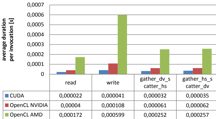
Figure 3. CUDA vs OpenCL I/O and communication for DL_POLY constraints shake component
